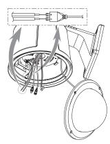
Connect the video cable, the controller cable, the camera power adapter cable and the ID setting cable to the speed dome camera.
